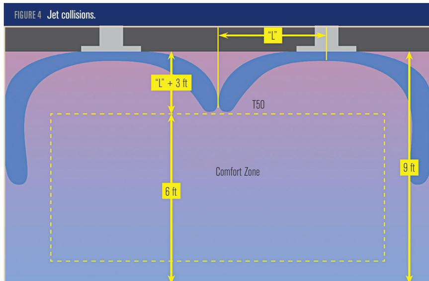
It is reduced the farther away the jet is from the air outlet. If the jet is cooler, and thus denser, than the room air, it will detach from the ceiling when the forward momentum of the supply jet is less than the downwards buoyancy force. If the buoyancy force is great enough, the supply jet may enter the occupied zone with an objectionable temperature or velocity. This effect is predictable and should be considered by the designer.
