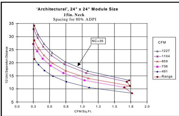
Figure 2 shows the performance of an Architectural (plaque) diffuser with a similar 4 jet pattern. Here one can see that this diffuser will both have better performance at low flows, and will have greater turn down in a VAV situation.
