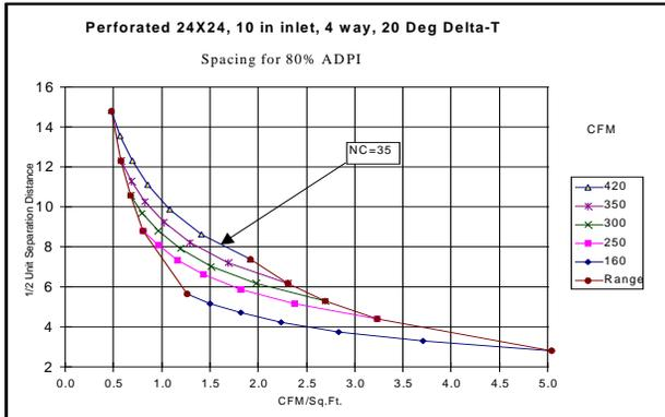
Figure 1 shows the performance envelope of a low cost perforated diffuser with a load resulting from a room/supply differential of  $20^{\circ}\Delta T$ . (Different delta-t's will result in different load rates, and will change the location of the vertical boundaries somewhat.)
