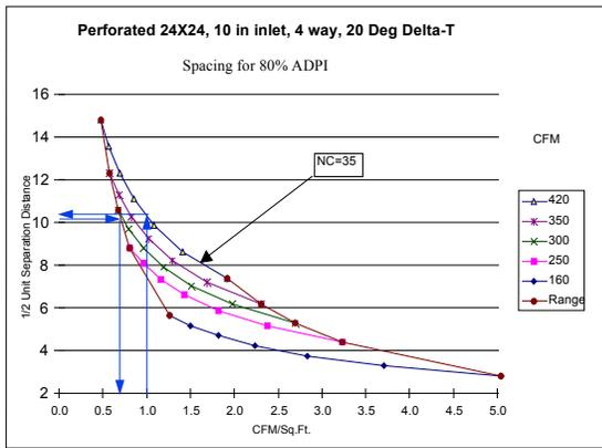
Figure 5: Selection using the envelope chart.
