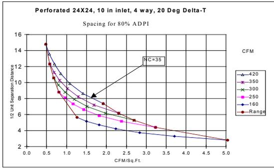
Figure 4: CFM/SqFt chart for a Perforated diffuser.
