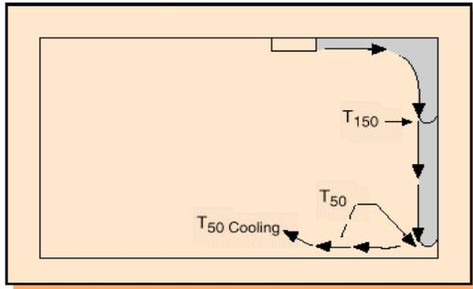
Figure 13: Diffuser directed at exterior wall.
