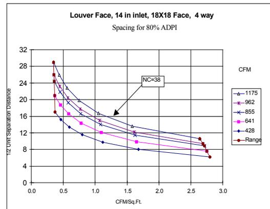
Figure 6: Louver Face Diffuser
